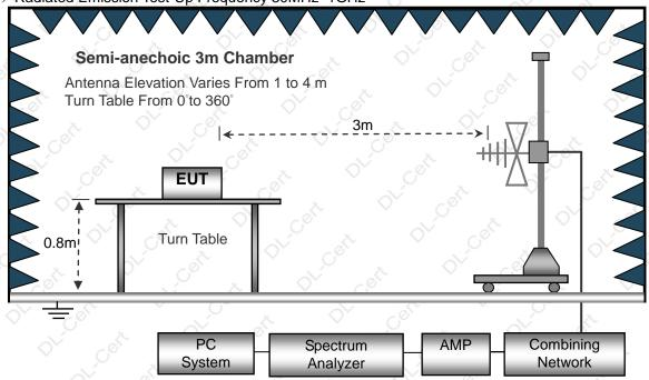
(C) Radiated Emission Test-Up Frequency Above 1GHz
