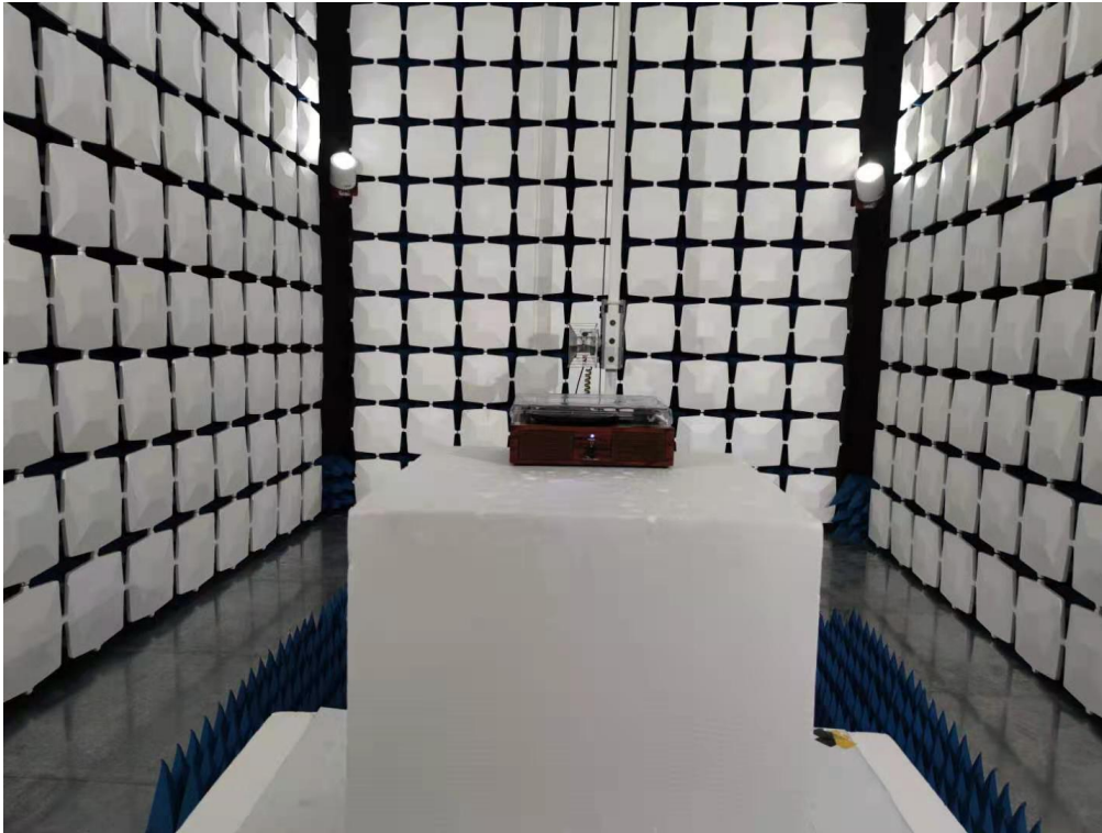
Above 1GHz for radiated emission test setup
