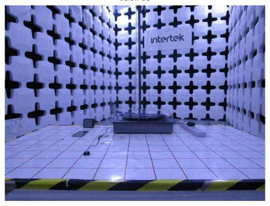
The EUT is Placed at the center of the Turntable.
