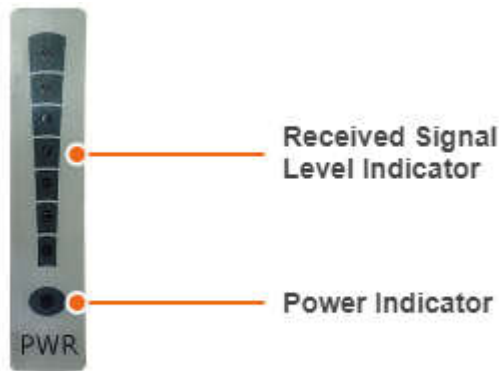
86 Figure - LED indication of InfiMAN Evolution ST, InfiLINK Evolution
