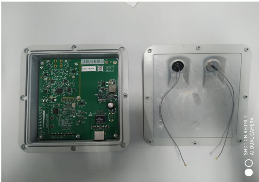
Internal view of E5-STE and cover with two connectors N type
