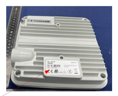
The label is placed on the side of the equipment enclose in a specially designated place
