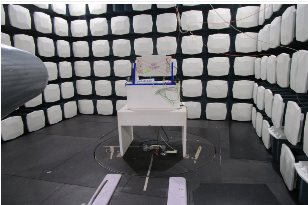
Photograph 4: EUT Test Setup in the fully anechoic chamber, Electric Field Strength
