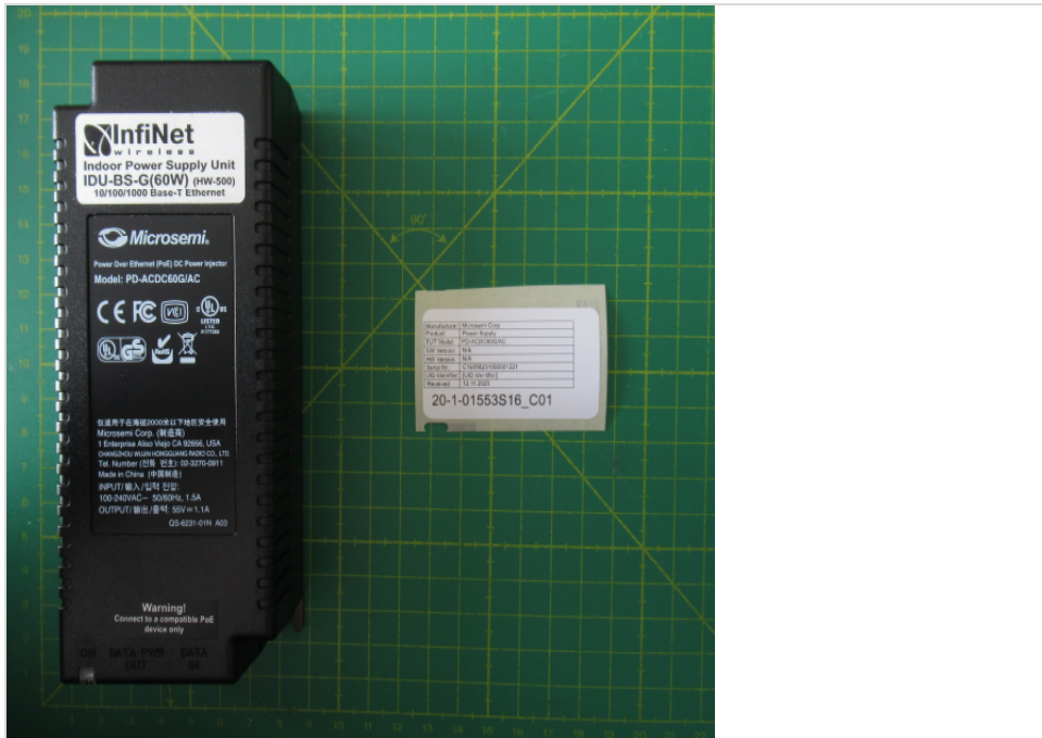
Photograph 3: AE2 Power Supply
