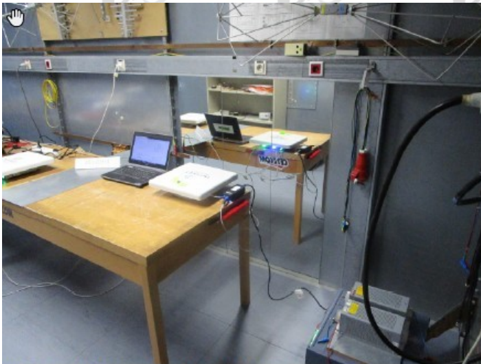
Photograph 3: Conducted emission test set-up
