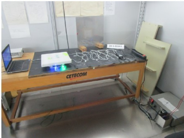
Photograph 9: Immunity test, test setup for ESD
