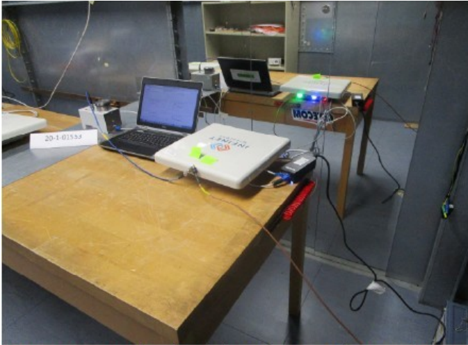
Photograph 4: Conducted emission test set-up , Telecommunication port
