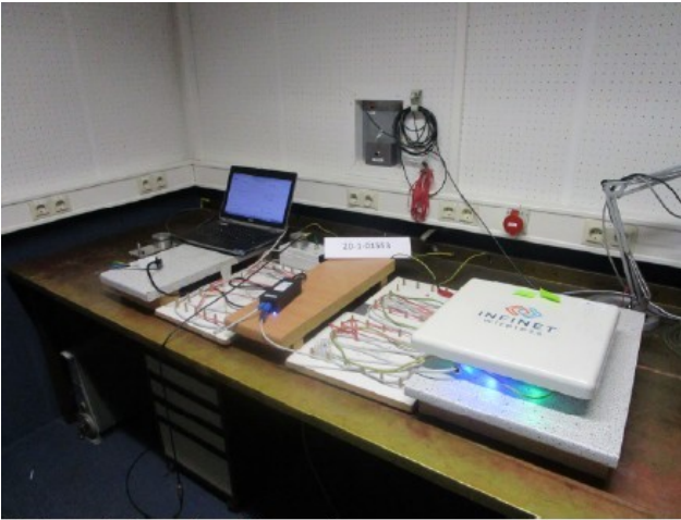
Photograph 5: conducted immunity test set-up
