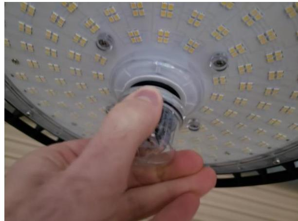
Power up the light fixture's main power and the auxiliary 12V power should power up your Z10 module.
