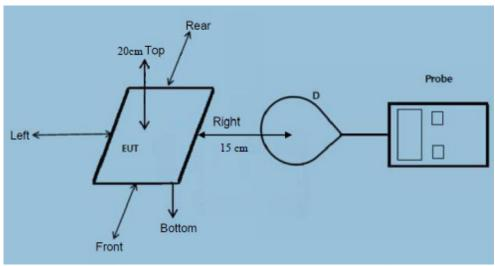
Remark: The E300 probe antenna diameter is less than 11.5cm.
