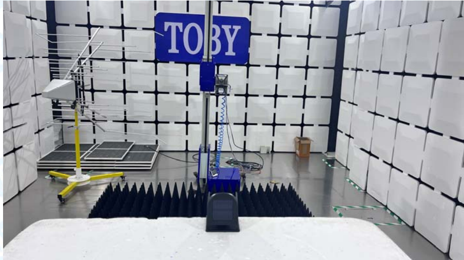
Photo of Setup for Radiated Emission (Above 1 GHz)
