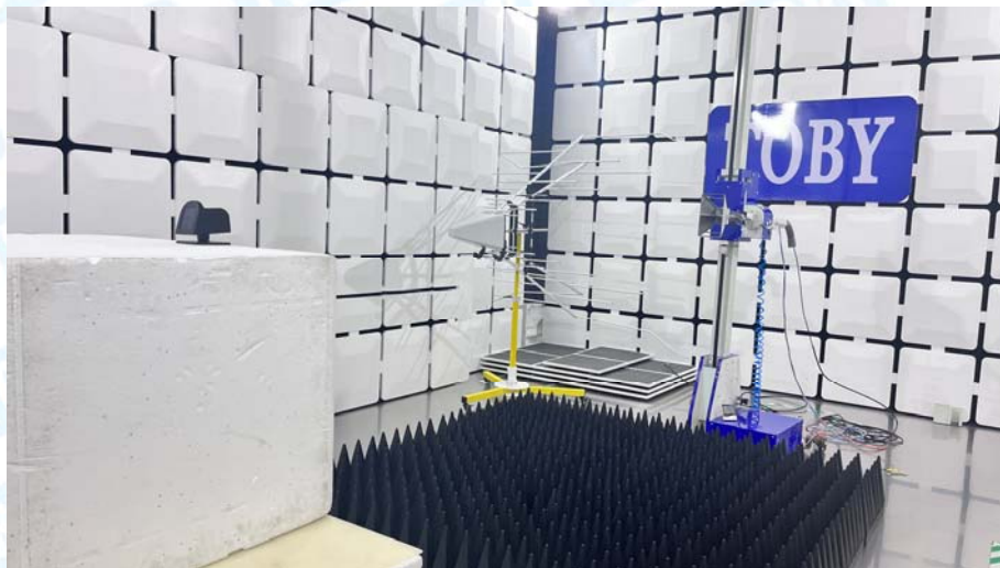
Photo of Setup for Radiated Emission (Above 1 GHz)
