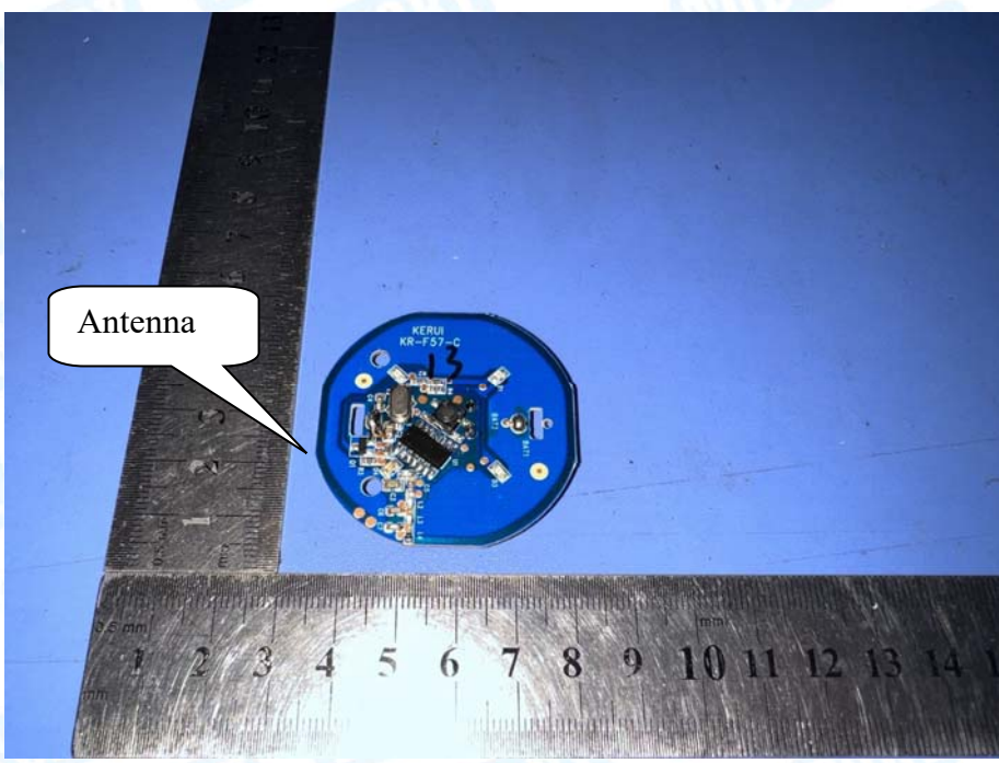
Photo 4 Internal of PCB
