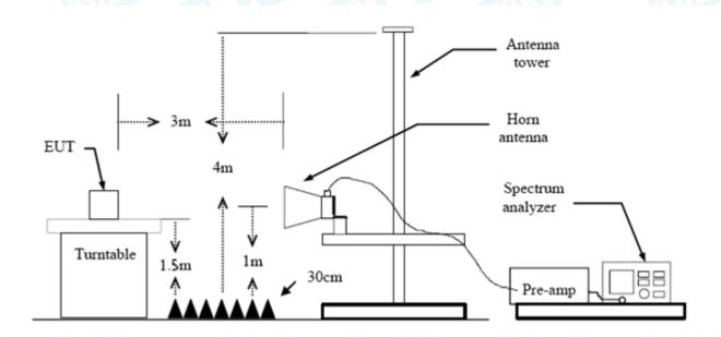
Above 1GHz Test Setup
