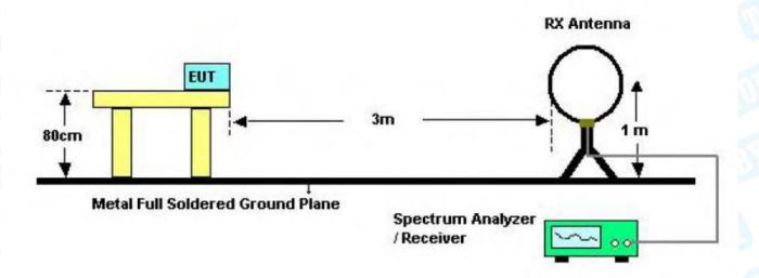
Below 30MHz Test Setup
