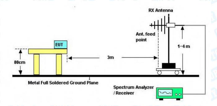
Bellow 1000MHz Test Setup
