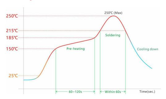
Please use the reflow within 2 times. Set up the highest temperature within 250℃.
