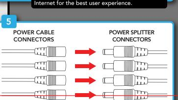
Connect the red female power leads of the video / power cables to the male power splitter ends.
