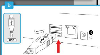
Plug the USB mouse into the USB port on the back of the DVR.
