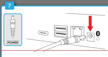
Connect the DVR power adapter to the Power Input on the rear of the DVR.
