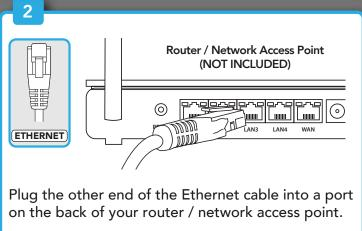
As long as your DVR is hardwired using Ethernet cabling, you can connect to any working network access point. See your product manual for more details.
