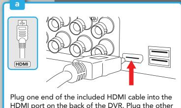
HDMI port on the back of the DVR. Plug the other end of the cable into your TV or Monitor.
