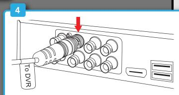
Connect the video / power cable labeled TO DVR ONLY to an open video input on the DVR.
