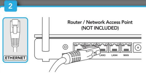
Plug the other end of the Ethernet cable into a port on the back of your router / network access point.
