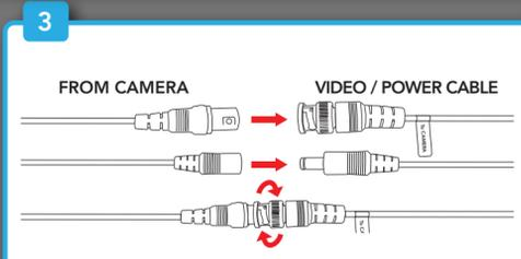
Connect the end of the camera's cable to the end of a video / power cable labeled TO CAMERA ONLY.
