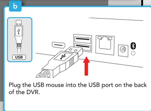
Plug the USB mouse into the USB port on the back of the DVR.
