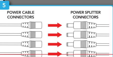
Connect the red female power leads of the video / power cables to the male power splitter ends.
