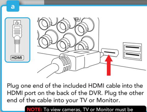
Plug one end of the included HDMI cable into the HDMI port on the back of the DVR. Plug the other end of the cable into your TV or Monitor.
