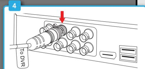
Connect the video / power cable labeled TO DVR ONLY to an open video input on the DVR.
