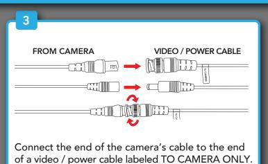
BEFORE installing, connect and test each camera locally to confirm they function properly.
