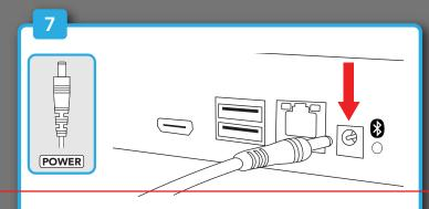
Connect the DVR power adapter to the Power Input on the rear of the DVR.
