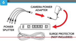
Connect the power splitter to the camera power adapter and plug the adapter into a surge protector or Uninterruptible Power Supply (UPS).
