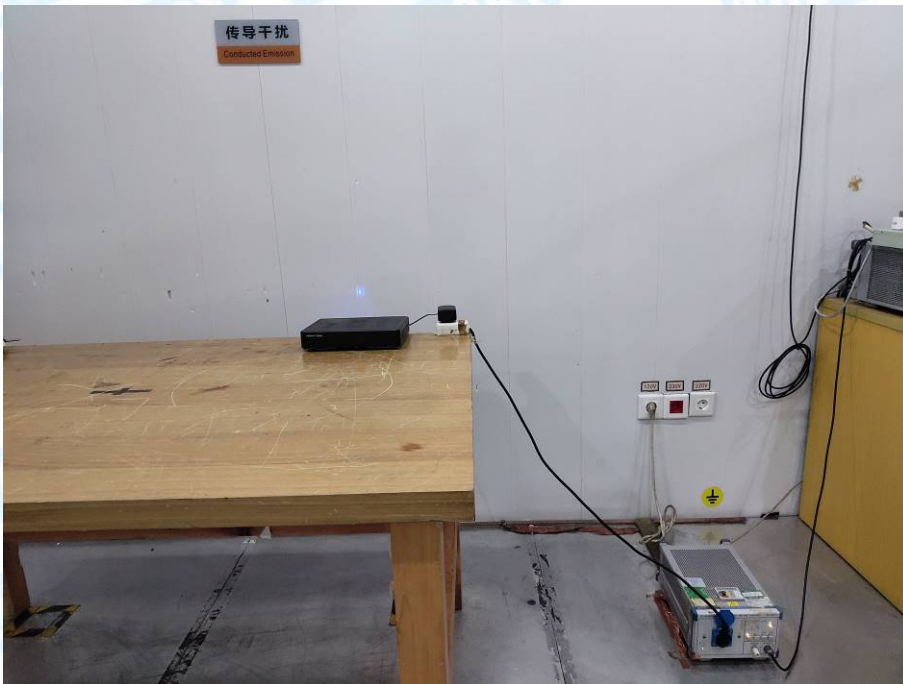
Photo of Setup for Conducted Emission
