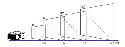
NOTE: Because the optical device has about 3% error, the above data is for reference only, please install the projector according to the actual measurement.
