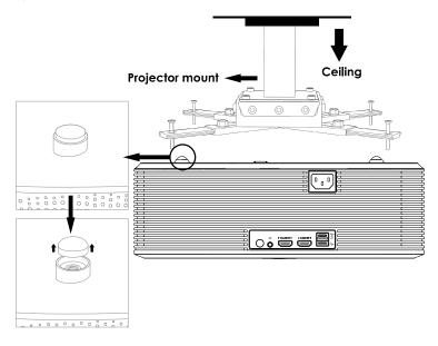
Fixed Hanger Screw Hole Type: 1/4 inch (M4\*4).
