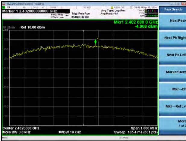
GFSK (BLE 1Mbps) LOW CHANNEL
