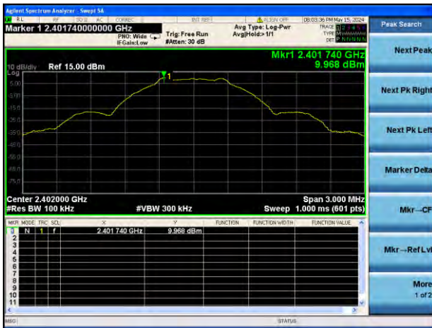
GFSK (BLE 1Mbps) LOW CHANNEL, CARRIER LEVEL
