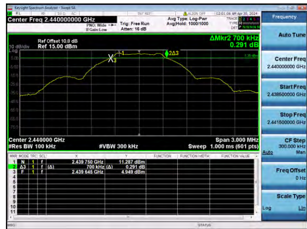
GFSK (BLE 1Mbps) MIDDLE CHANNEL
