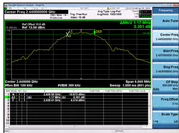
GFSK (BLE 2Mbps) MIDDLE CHANNEL
