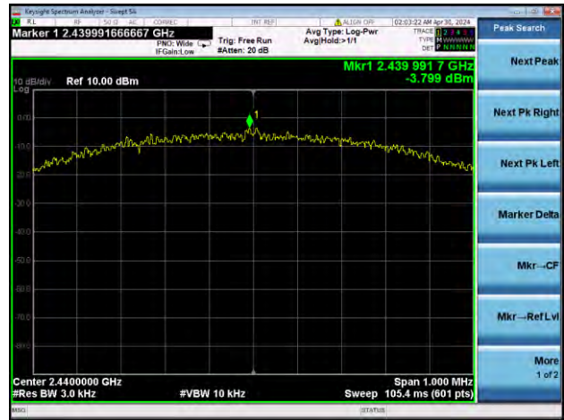
GFSK (BLE 1Mbps) MIDDLE CHANNEL
