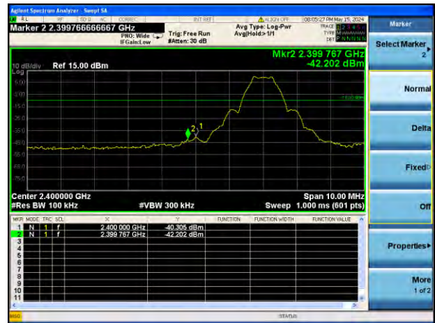
GFSK (BLE 1Mbps) HIGH CHANNEL, BAND EDGE
