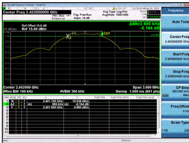
GFSK (BLE 1Mbps) LOW CHANNEL
