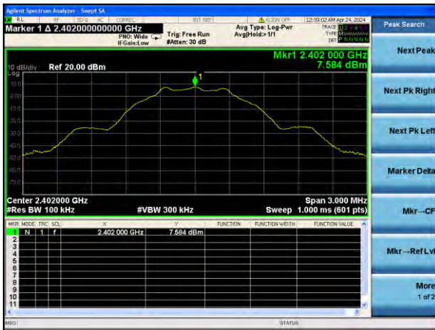
GFSK (BLE 1Mbps) LOW CHANNEL, CARRIER LEVEL
