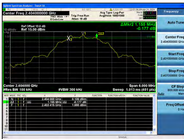
GFSK (BLE 2Mbps) LOW CHANNEL
