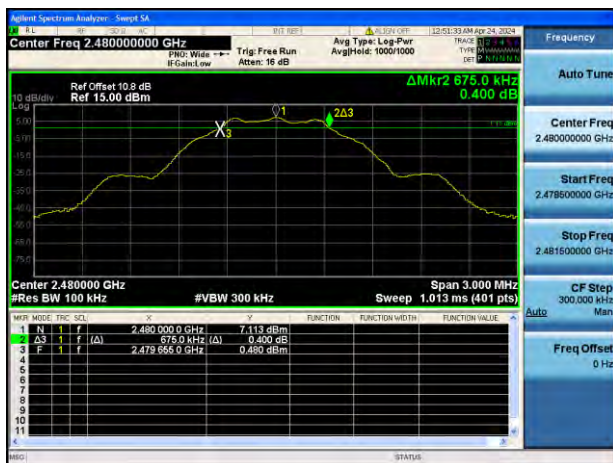
GFSK (BLE 1Mbps) HIGH CHANNEL
