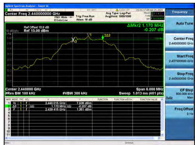
GFSK (BLE 2Mbps) MIDDLE CHANNEL
