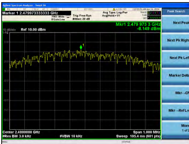
GFSK (BLE 1Mbps) HIGH CHANNEL
