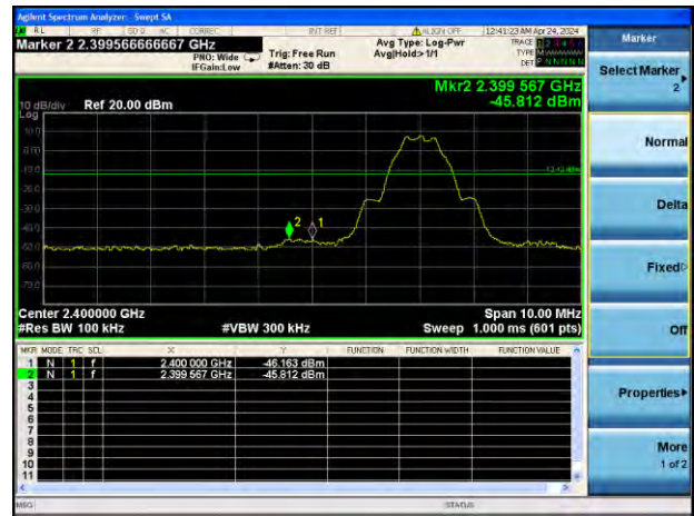
GFSK (BLE 1Mbps) HIGH CHANNEL, BAND EDGE
