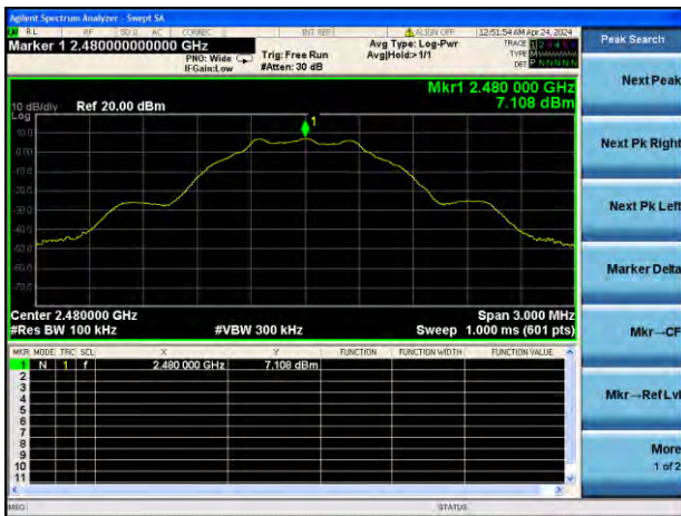
GFSK (BLE 1Mbps) HIGH CHANNEL, CARRIER LEVEL
