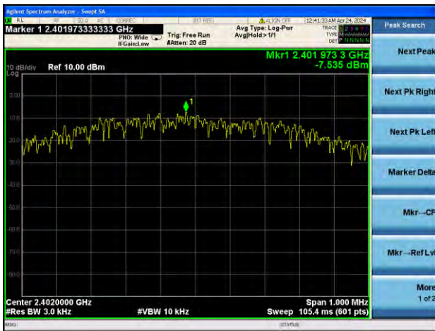
GFSK (BLE 1Mbps) LOW CHANNEL
