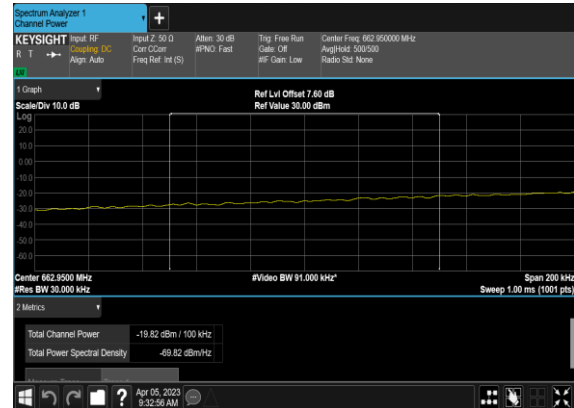
N71(10M)_DFT-s- OFDM_QPSK_Edge_1RB_Left_Low_CH_CHP_PA SS
