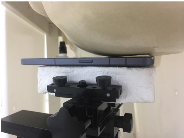
Left Cheek, Test Separation 0 mm
