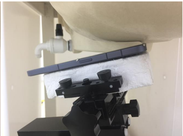
Left Tilted, Test Separation 0 mm
