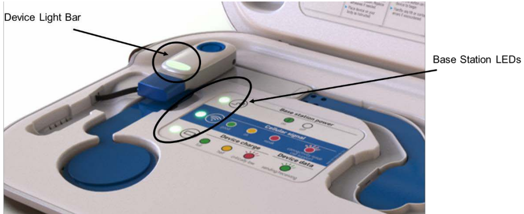
Figure 24. Locations of the light bar on the CPM Device and Base Station LEDs.
