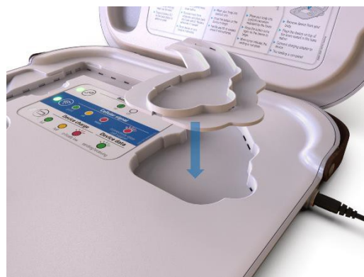
Figure 17. Inserting the correct adjustment plate into the Base Station
