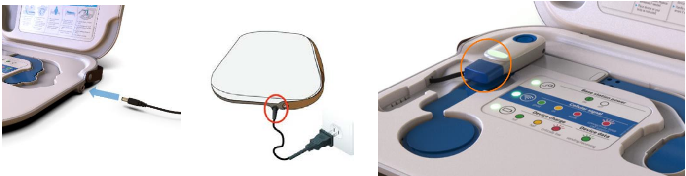
Figure 22 a-c. a-b) Plugging the Base Station into the wall and c) Magnetic charging and LED indications in the Base Station.
