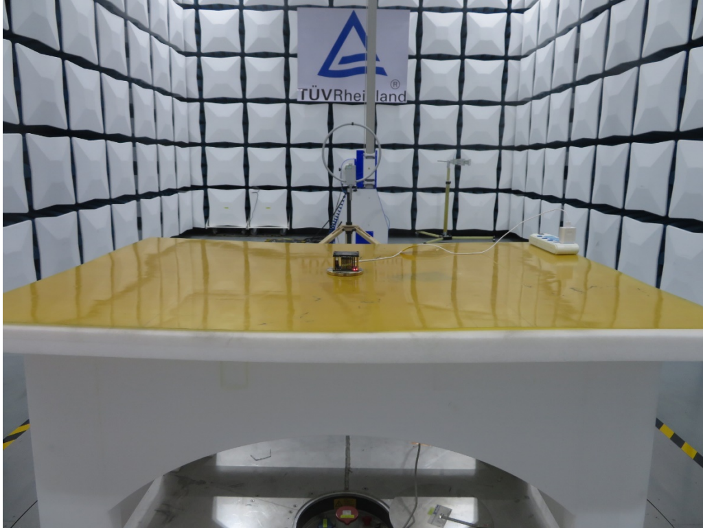
Photograph 2: Set-up for Radiated Spurious Emissions, above 30MHz
