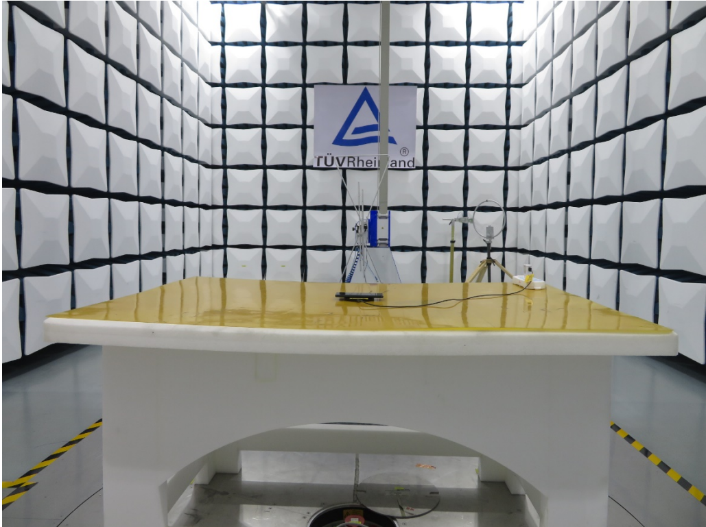
Photograph 2: Set-up for Radiated Spurious Emissions, above 30MHz
