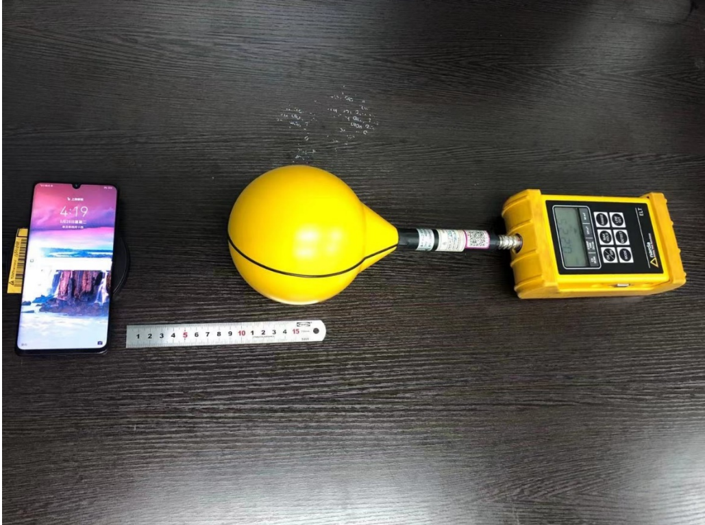
Photograph 5: Set-up for RF Exposure
