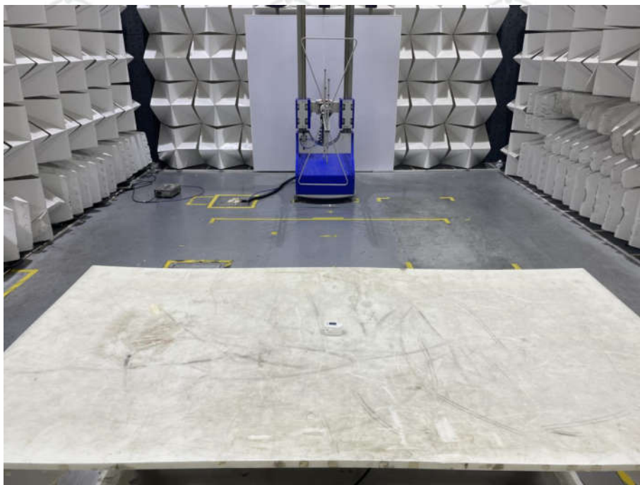
Radiated spurious emission Test Setup-1(Below 1GHz)
