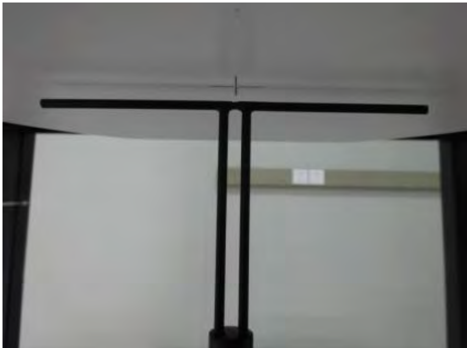
Photo of Dipole Setup
