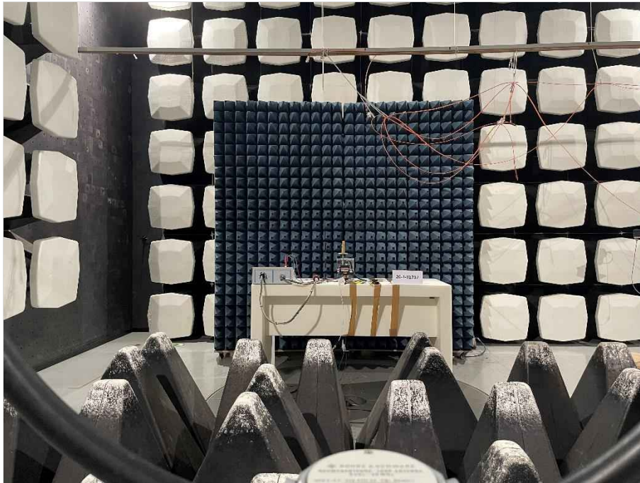
Photograph 7: EUT Test Setup in the semi anechoic chamber, close up view_EUT elevation 90°
