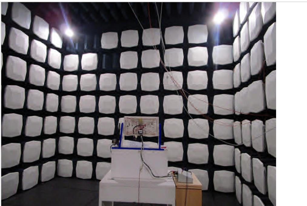
Photograph 4: EUT test setup in the fully anechoic chamber, overview
