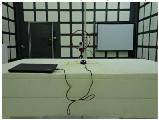
Radiated Emission Set up Photos (Below 1GHz)
