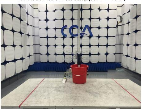
Radiated emission Test Setup (30MHz~1GHz)
