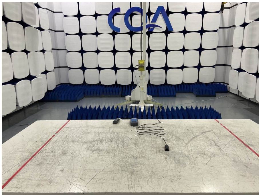
Radiated emission Test Setup (Above 1GHz)
