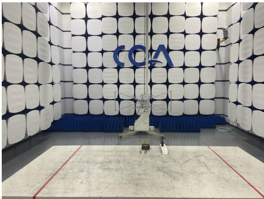
Radiated emission Test Setup (30MHz~1GHz)
