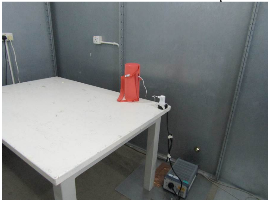
Measurement of Conducted Emission Test Set Up
