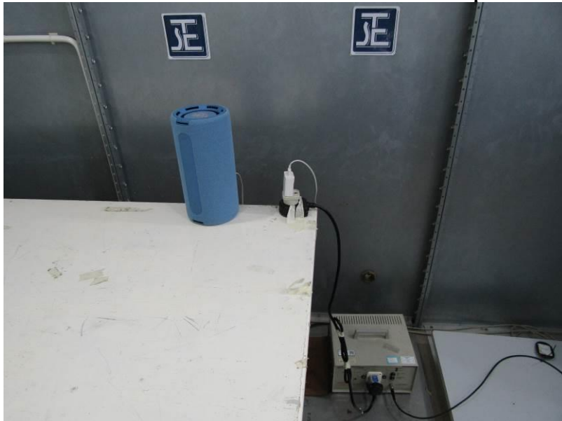
Measurement of Conducted Emission Test Set Up
