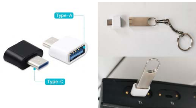
Figure 3.7.10 Connection diagram of mobile storage device
