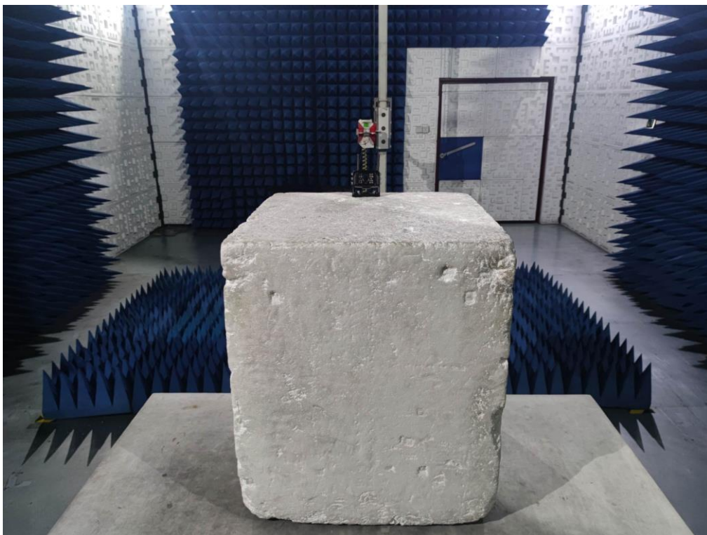
RADIATED EMISSION TEST SETUP ABOVE 1GHz
