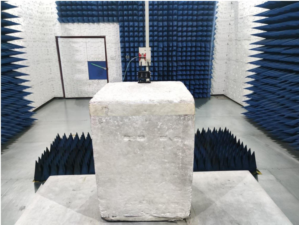
FCC RADIATED EMISSION TEST SETUP ABOVE 1GHZ
