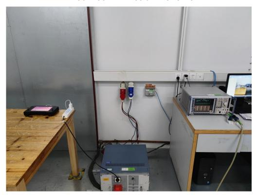
RADIATED EMISSION TEST SETUP BELOW 1GHZ
