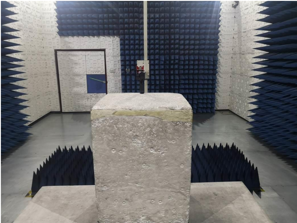
FCC RADIATED EMISSION TEST SETUP ABOVE 1GHZ
