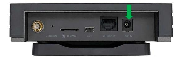
Insert a pin into the BT BUTTON hole and press the button for 5 seconds, and then
