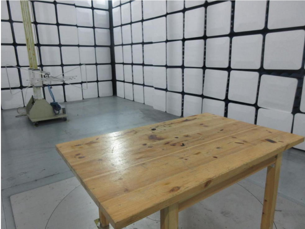
FCC ID: 2AZC8-BT4 Photo of Radiation Emission Test
