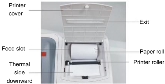
Inner structure of the printer
