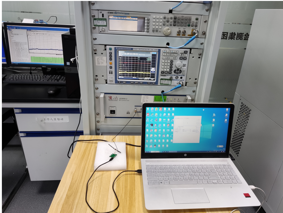
CONDUCTED EMISSION TEST SETUP
