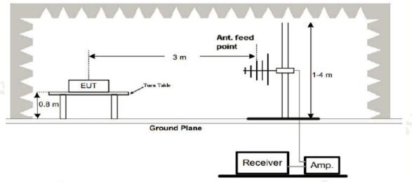
3. Radiated Emission Test-Up Frequency Above 1GHz
