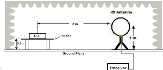
2. Radiated Emission Test-Up Frequency 30MHz~1GHz
