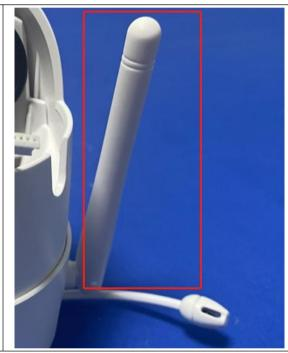
The antenna is External antenna. The best case gain of the antenna is 3dBi.
