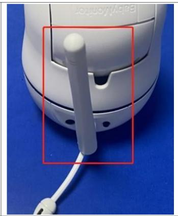
The antenna is External antenna. The best case gain of the antenna is 0dBi. The antenna is permanently connected, any removal will render the antenna inoperable.
