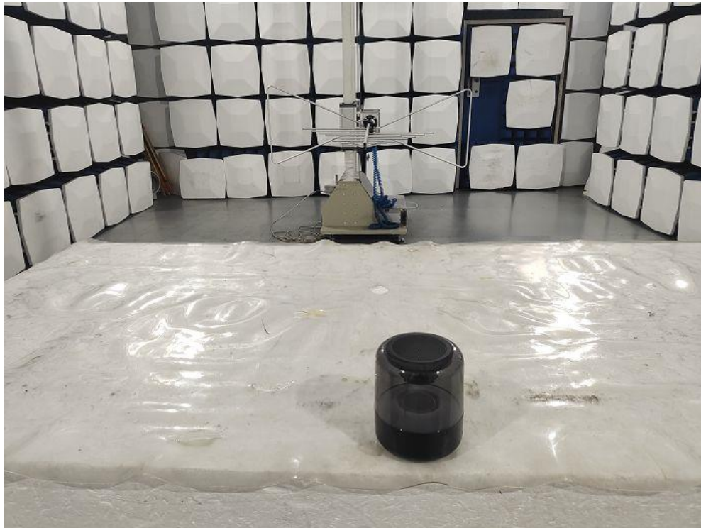
Radiated Emission Test Setup:
